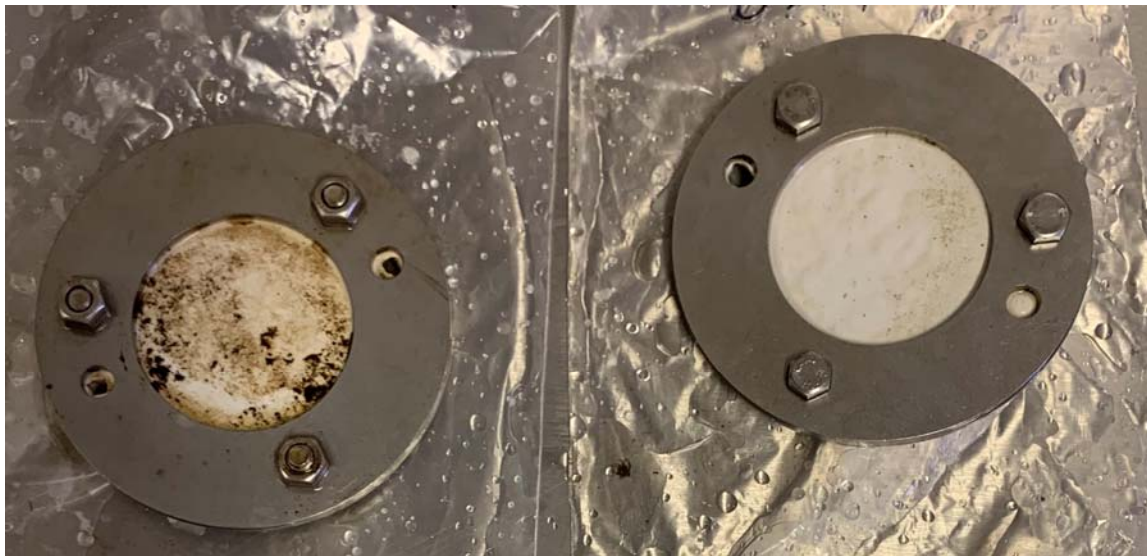
Plate 6: POCIS passive samplers following retrieval
