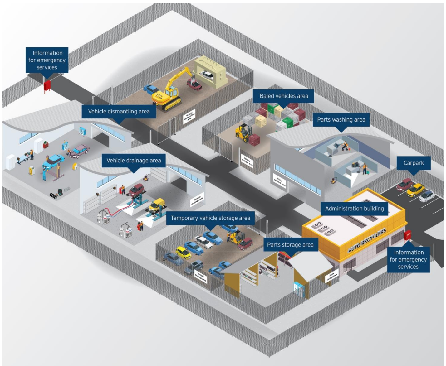
Figure 3: Site plan showing different work areas typically found in an auto recycling work site
