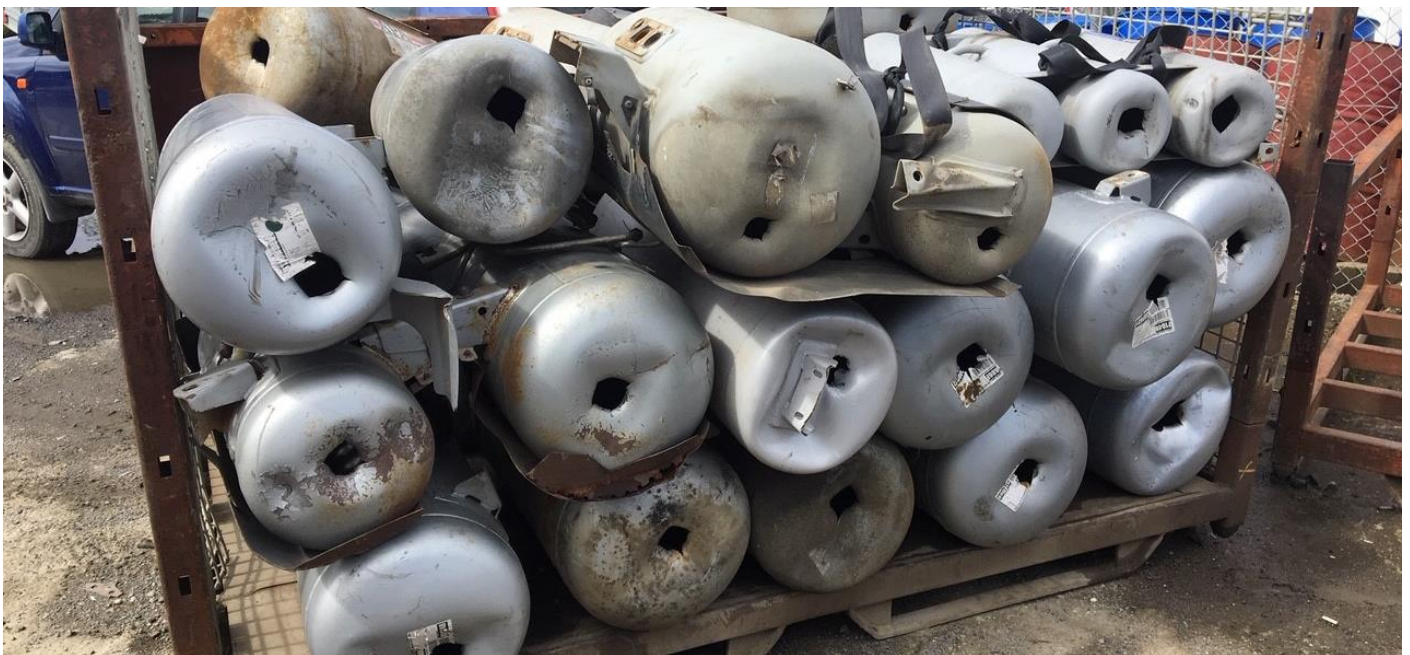
Figure 8: Pierce gas cylinders as an indication to the scrap metal collector that they are empty of content.
