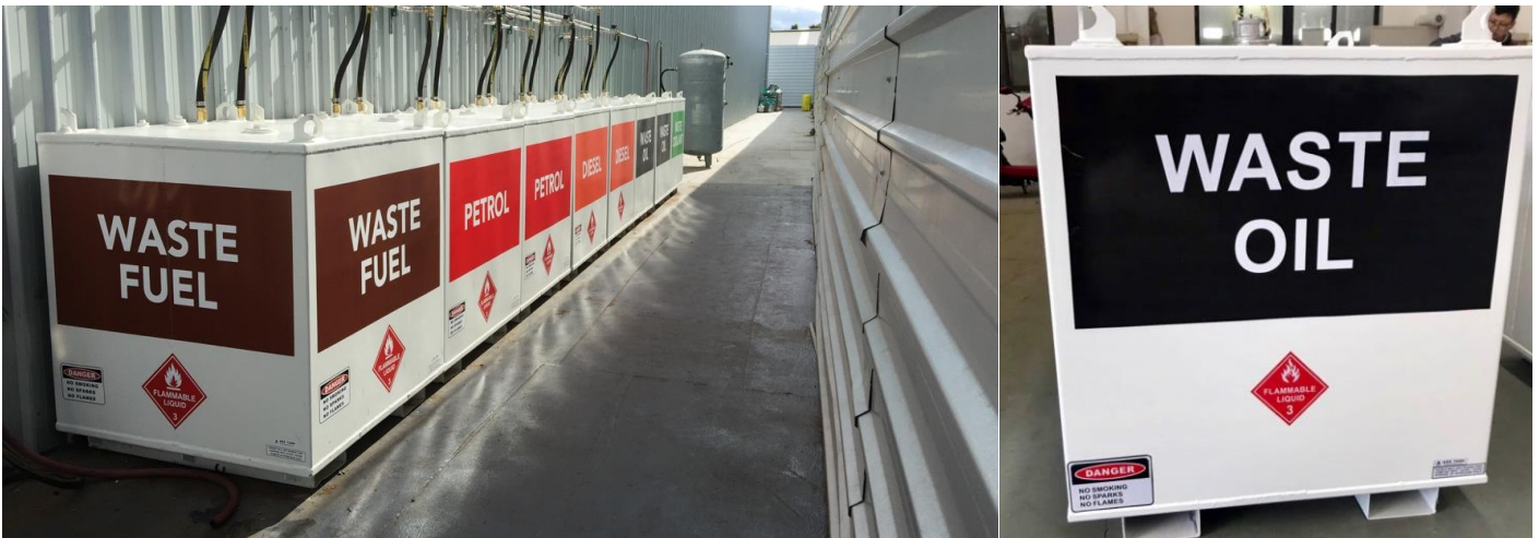
Figure 5: Clearly labelled waste oil and other liquid containers at an auto recycling site
