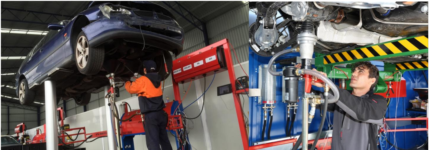
Figure 7: Collecting fuel from the end of life vehicles
