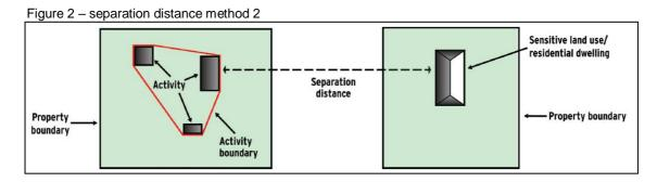
This method may be appropriate where there are only a few sensitive receptors, usually in rural settings, which are located outside of a sensitive land use zone and the activity area will not change. The distance required for odour dispersion should be within the property boundary of the facility.
