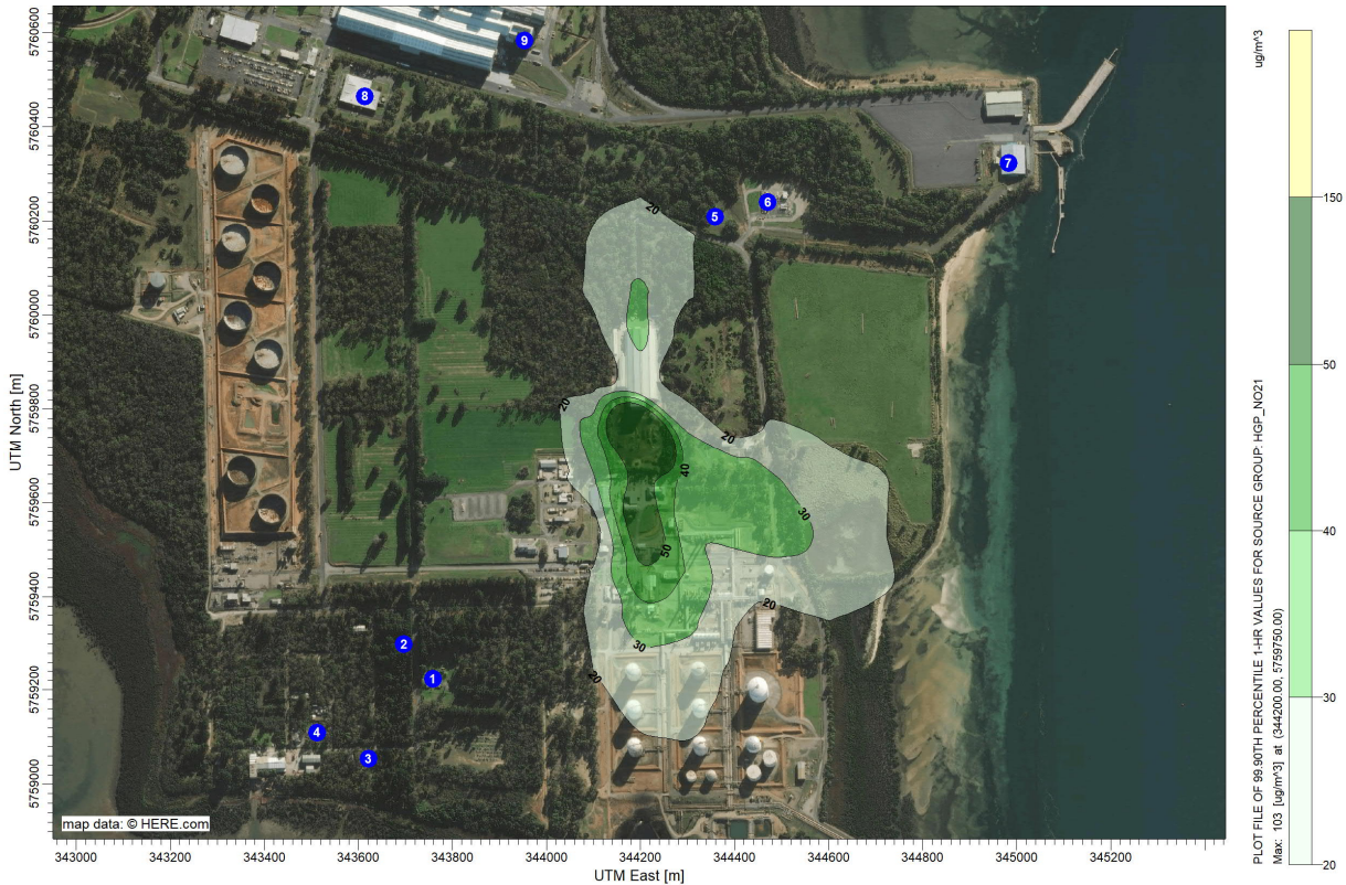
Figure 11 NO 2 results, Hasting power generation Project with 100ppm emissions, 1-hr average 99.9 th percentile, no background, 2016 MET ( \mu\text{g}/\text{m}^3 )
