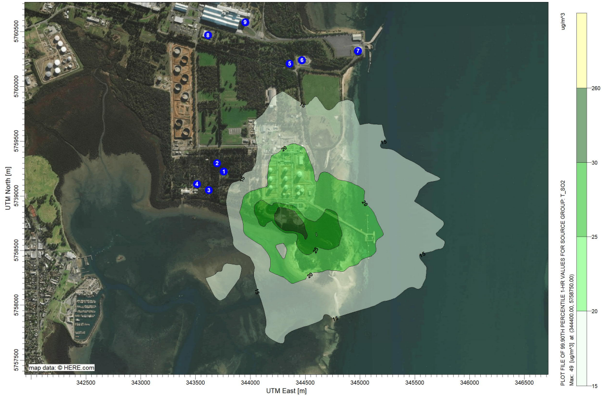
Figure 18 SO 2 results, Hasting power generation Project and LIP emissions, 1-hr average 99.9 th percentile, no background, 2016 MET (µg/m 3 )
