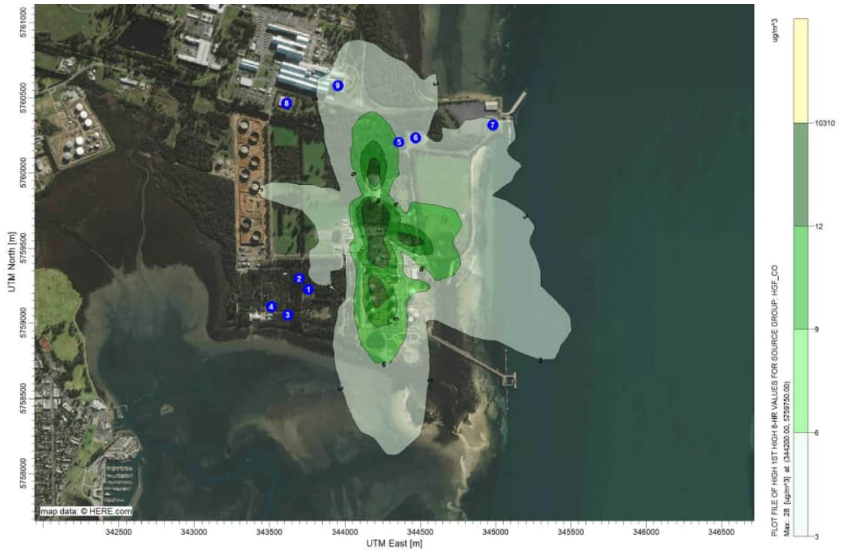
Figure 15 CO results, Hasting power generation Project emissions, maximum 8-hr average, no background, 2016 MET ( \mu\text{g}/\text{m}^3 )
