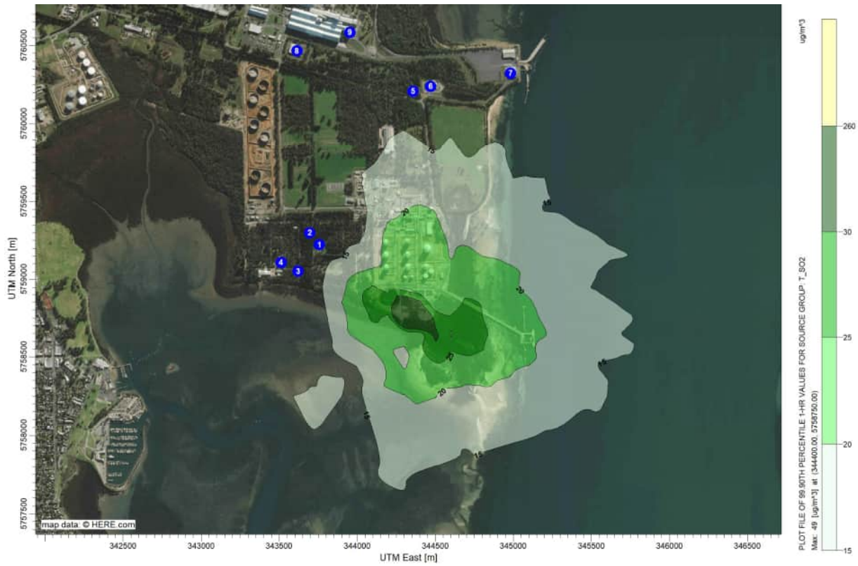
Figure 18 SO 2 results, Hasting power generation Project and LIP emissions, 1-hr average 99.9 th percentile, no background, 2016 MET ( \mu\text{g}/\text{m}^3 )
