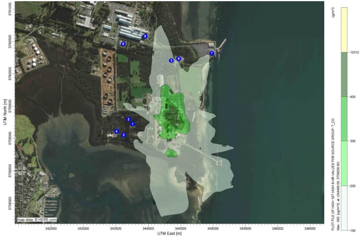
Figure 17 CO results, Hasting power generation Project and LIP emissions, maximum 8-hr average, no background, 2016 MET ( \mu\text{g}/\text{m}^3 )
