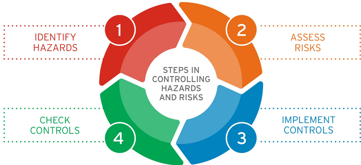
Figure 1: Steps in controlling hazards and risks
