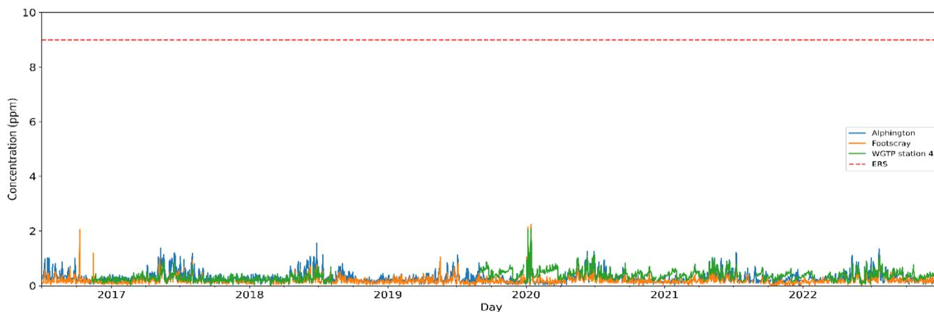
**Figure 6.** 8-hourly averaged CO concentrations measured at EPA stations (Alphington and Footscray) and WGTP 4. Note: in 2017, CO data is available from 05 January to 31 December at WGTP4.
