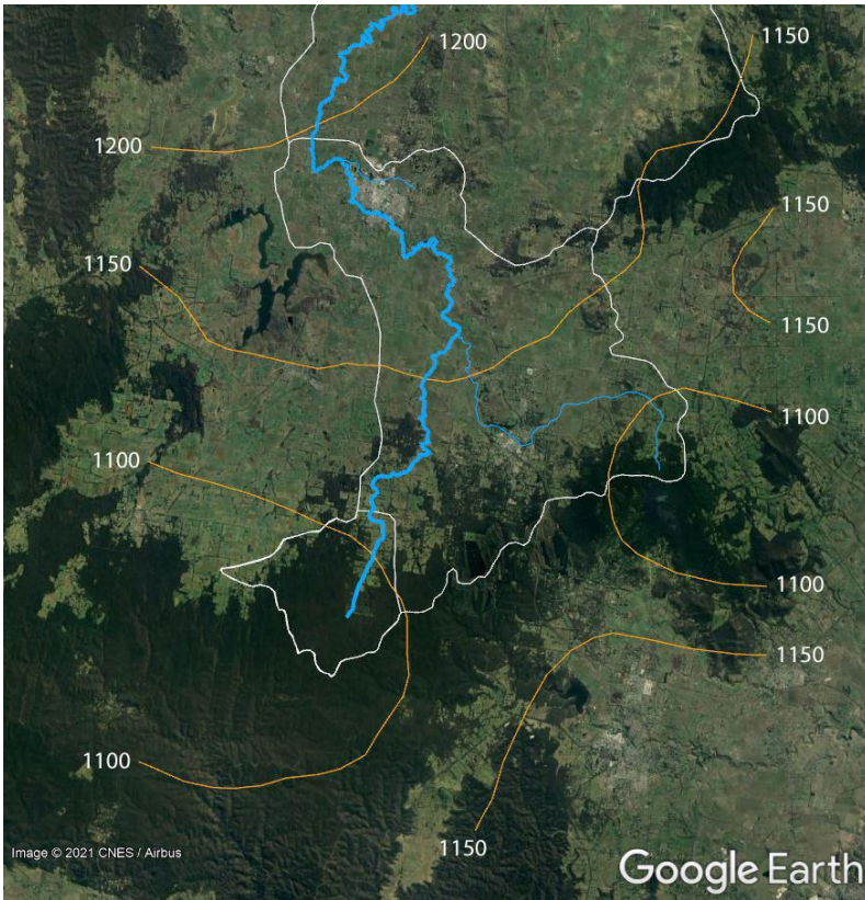
Figure 10 Average annual pan evaporation (mm) for the upper Campaspe River (source: SILO data)
