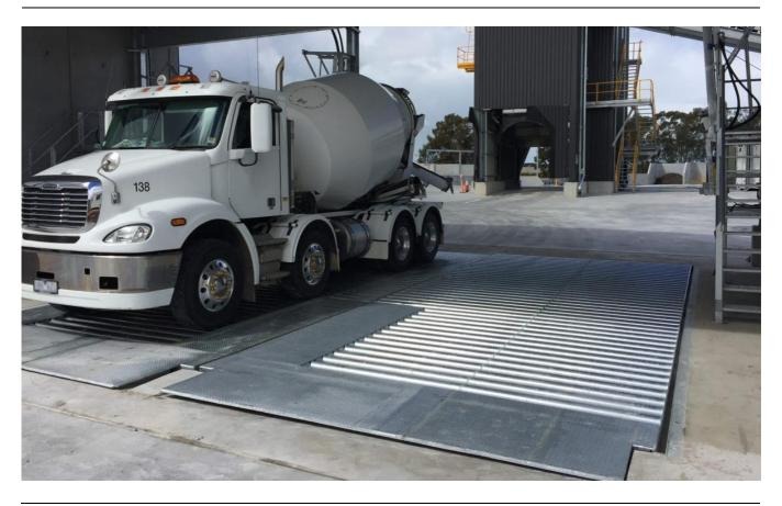
Figure 6. Slump station with grated floor to capture washwater for recycling back into production. Source: Cement Concrete and Aggregates Australia (CCAA).
