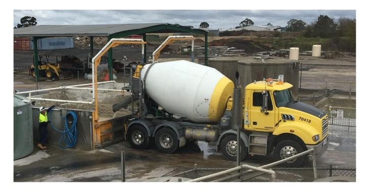
Figure 8. Waste concrete returned to batching plant for reclamation and recycling. Source: Cement Concrete and Aggregates Australia (CCAA).
