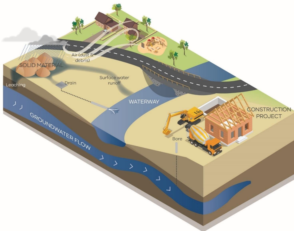
Figure 3.2. How pollution and waste from your activities can impact humans and the environment.
