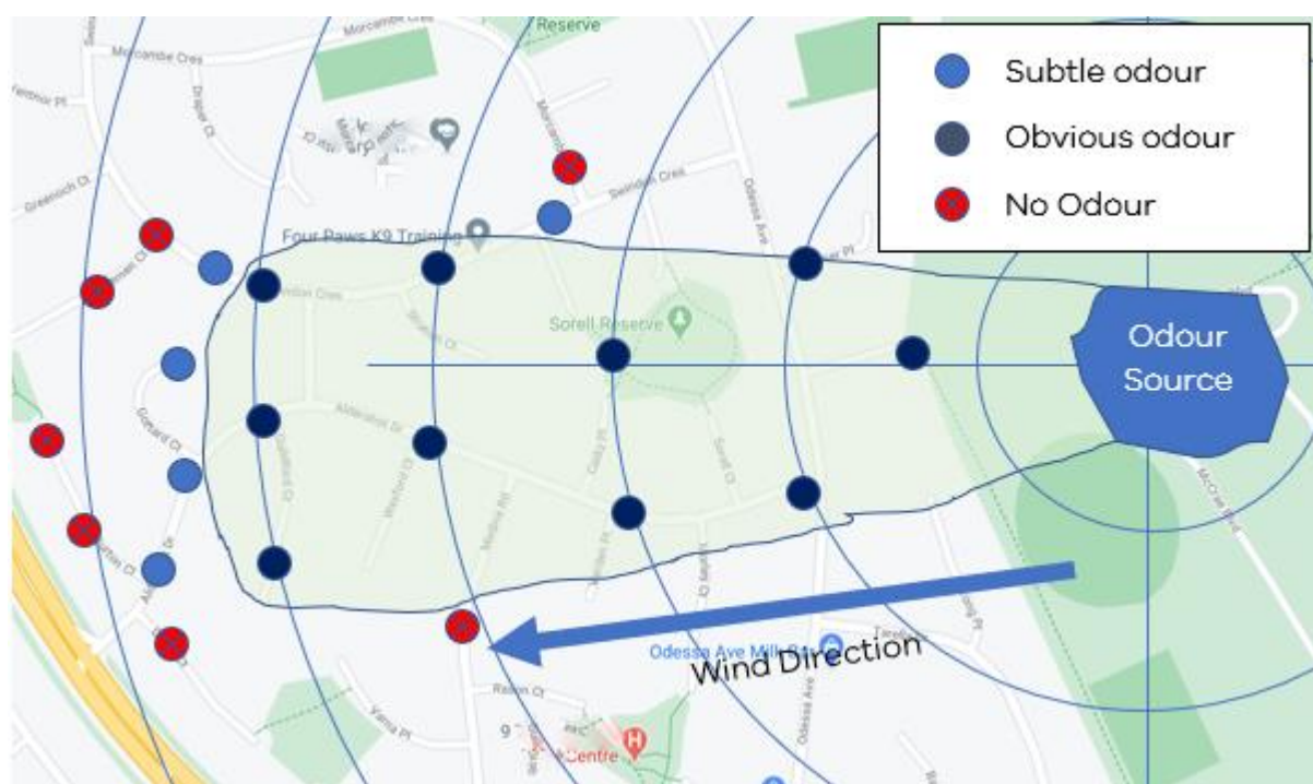
Figure 7: Example of a plume odour trace where car was used to locate the plume and more detailed odour observations made on foot.
