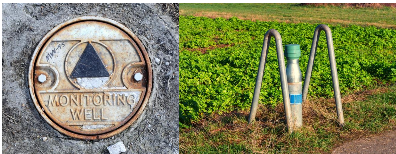
Figure 1: While not necessarily an indicator of contamination, the presence of groundwater wells generally indicates that groundwater has been assessed. An access cover (on left) and a standpipe (on right).
