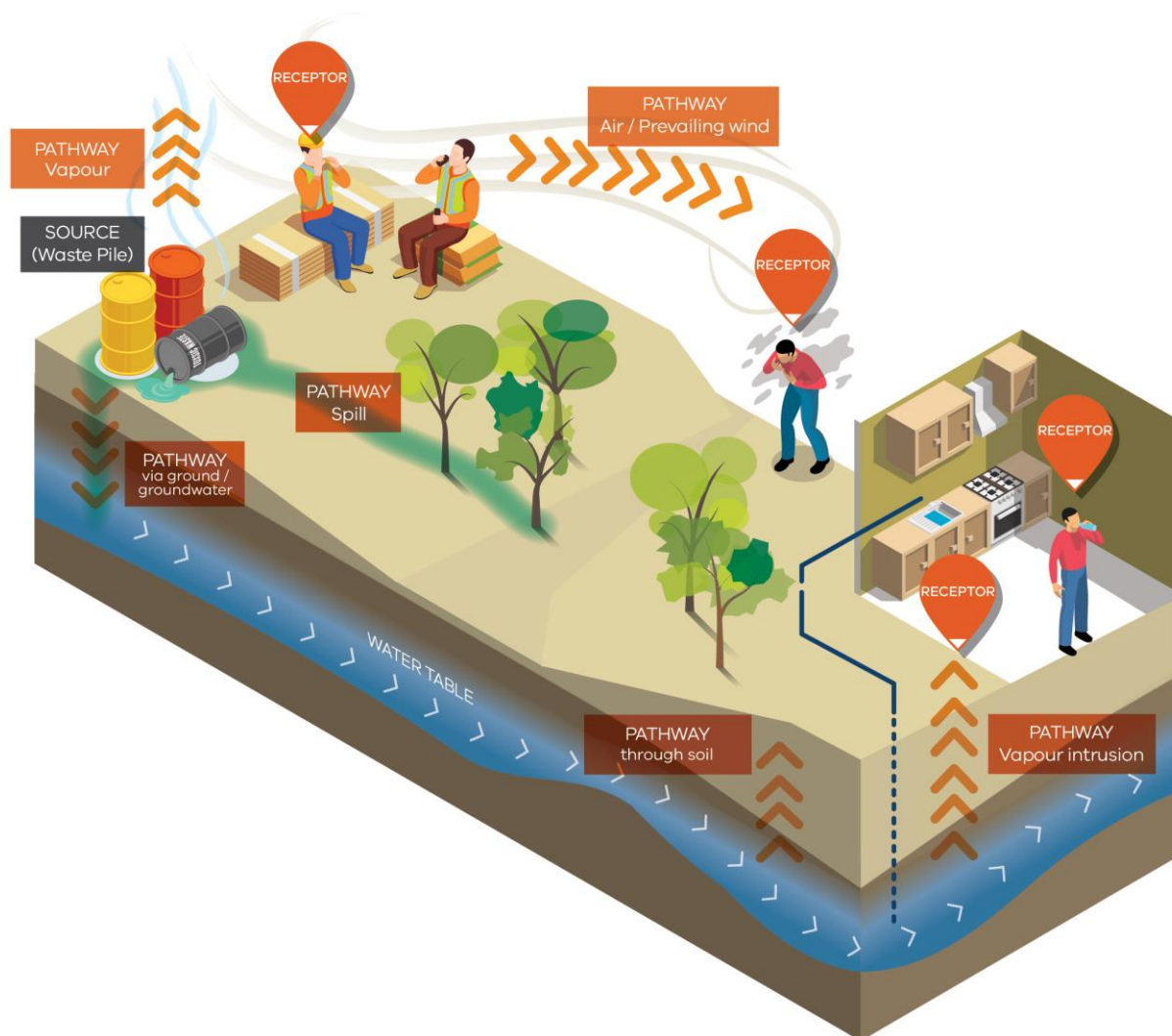
Figure 5: Conceptual site model shows how contamination can travel through ground, water and air (pathways) to cause harm to human health and the environment (receptor).
