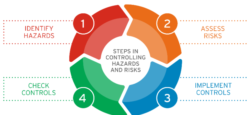
Figure 1: Steps in controlling hazards and risks
