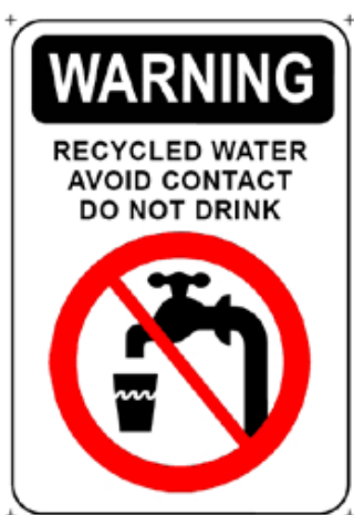
Figure 8-1: Example of recycled water warning signage
