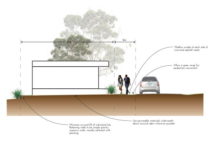
Diagram 6: Typical cross-section through cabin site
