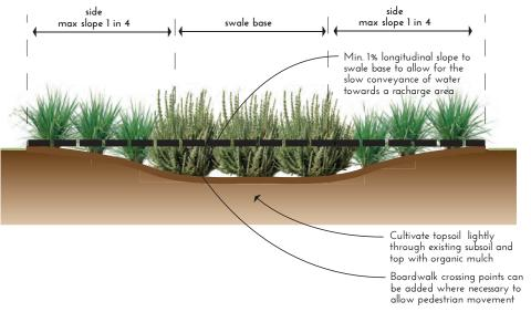
Diagram 9: Typical planted swale with conveyance
