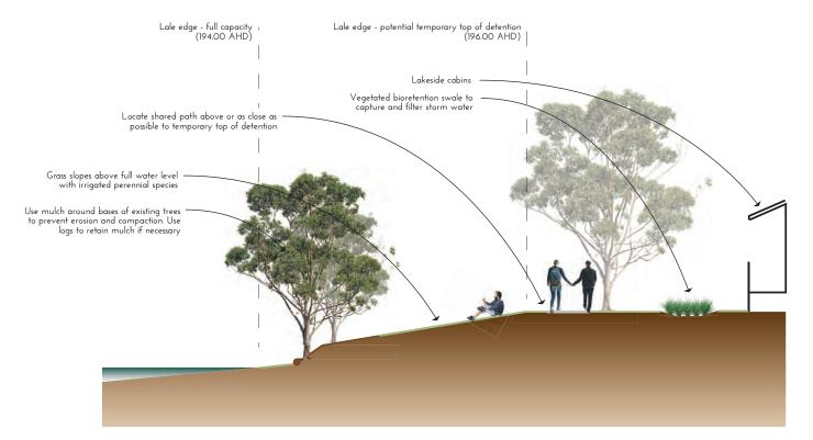
Diagram 7: Typical cross-section through foreshore area
