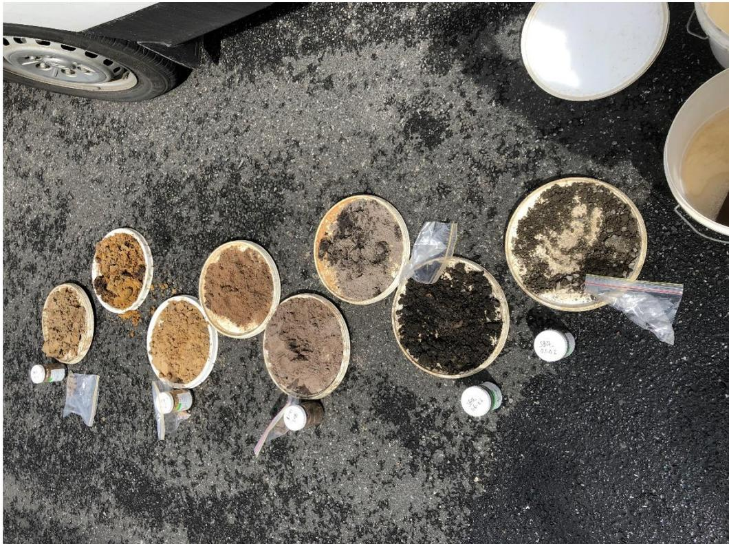
**Photo 14. SB7377 Lithology. Depth profile from right to left.**
