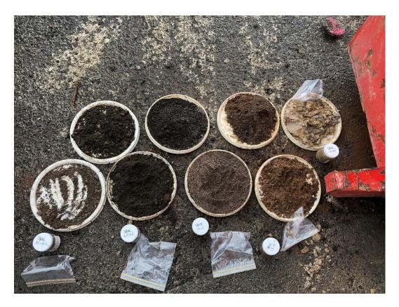
Photo 17. SB7378 Lithology. Depth profile from bottom left to top right.
