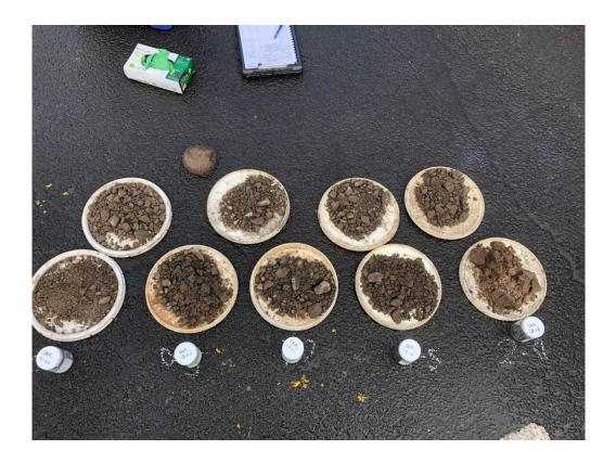
Photo 20. SB7379 Lithology. Depth profile from bottom left to bottom right.
