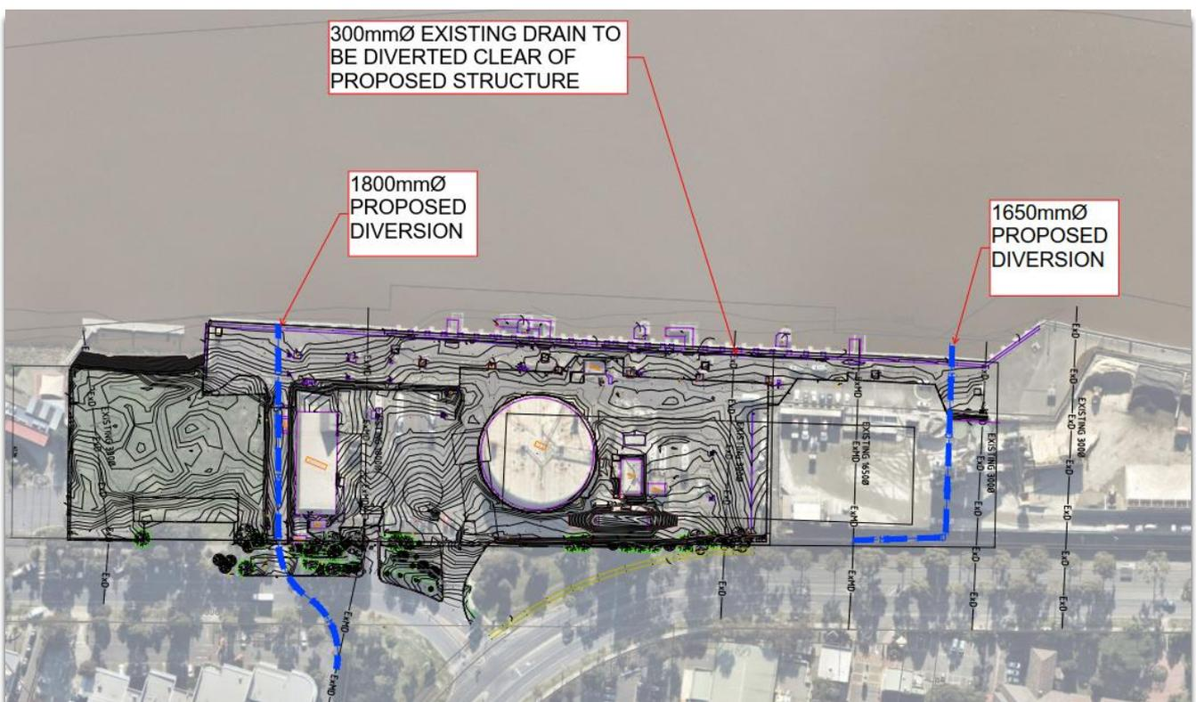
Figure 4 – Existing main drains and proposed diversion
