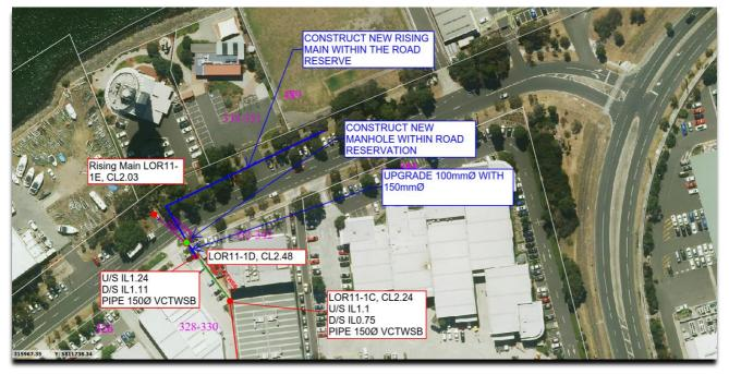
Figure 3 – Proposed Sewer Rising Main to Existing manhole LOR11-1D
