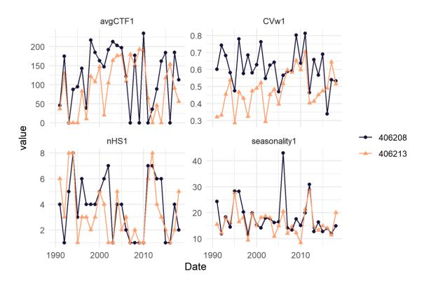
Figure 3. Key flow metrics in the upper Campaspe River calculated from daily flow data from gauges in the upper (406208) and lower (406213) reaches.
