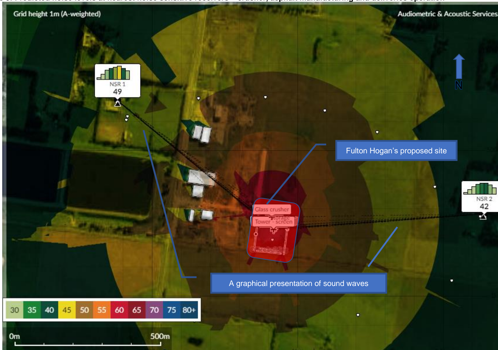
Figure 5: Predicted noise levels at nearest noise sensitive receivers – crusher, asphalt manufacturing and deliveries operation
