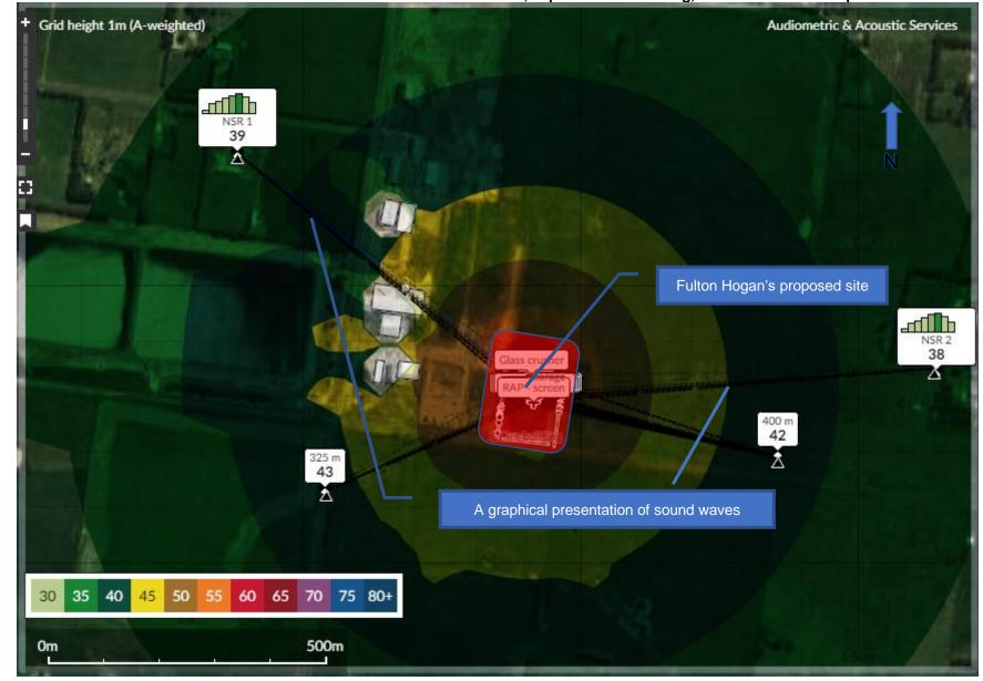
Figure 7: Predicted noise levels at nearest noise sensitive receivers – crusher, asphalt manufacturing, RAP and deliveries operation
