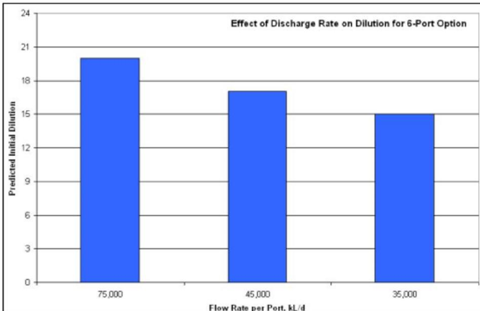
It is apparent that the discharge from the three trains must be directed to specific discharge ports, to maintain the high velocity discharge required to achieve high dilution.
