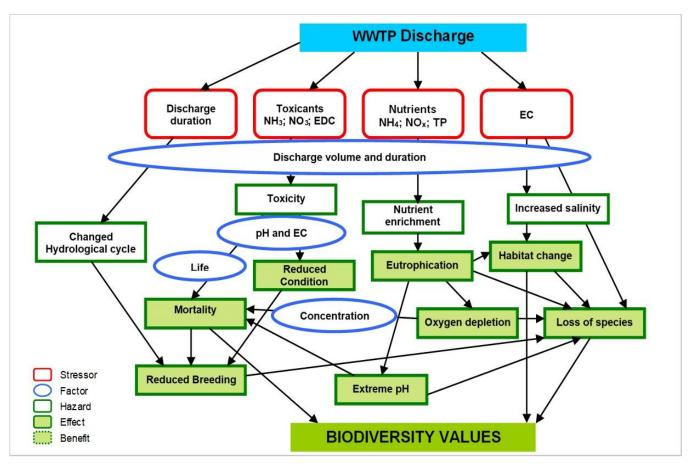
Figure B3 – Conceptual model of the relationship between a wastewater treatment plant (WWTP) discharge and the biodiversity values of the Goulburn River. Notes: EC = electrical conductivity, EDC = endocrine disruptive chemicals, NH<sub>3</sub> = ammonia, NH<sub>4</sub> = ammonium, NO<sub>3</sub> = nitrate, NO<sub>x</sub> = nitrogen oxide, TP = total phosphorus
