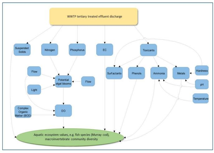
Figure A1 – Simplified conceptual model of the potential risks to a river aquatic ecosystem from a tertiary treated wastewater treatment plant (WWTP) effluent. Notes: DO = dissolved oxygen, EC = electrical conductivity, BOD = biological oxygen demand
