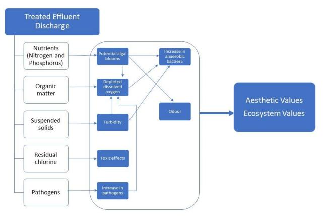
Figure B8 – Conceptual model of the interactions of ecosystem and aesthetic values with a small wastewater treatment plant discharge
