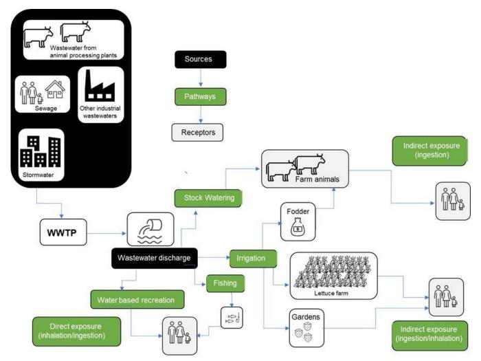
Figure C3 – Schematic diagram of the exposure pathways for a wastewater treatment plant
