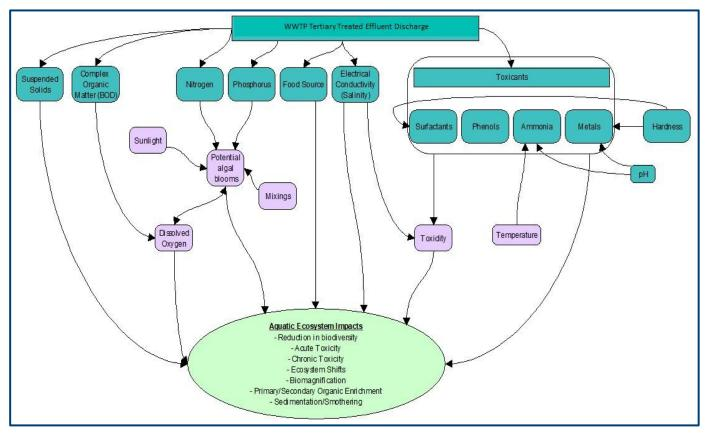
Figure B2 – Conceptual model of the direct interactions of a wastewater treatment plant (WWTP) discharge with a marine aquatic ecosystem
