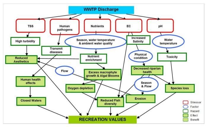
Figure B4 – Conceptual model of the relationship between a wastewater treatment plant (WWTP) discharge and the recreational values of the Goulburn River. Notes: EC = electrical conductivity, TSS = total suspended solids
