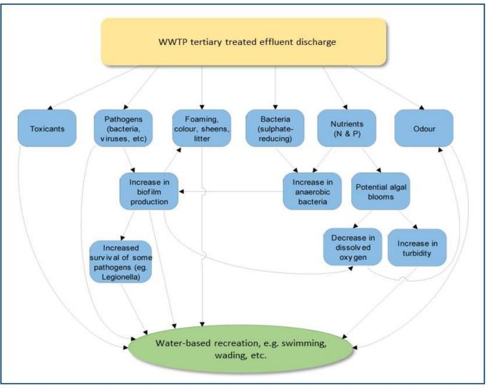
Figure A2 – Simplified conceptual model of the potential risks to the environmental value of water-based recreation from a tertiary treated wastewater treatment plant (WWTP) effluent. Notes: N = nitrogen, P = phosphorus
