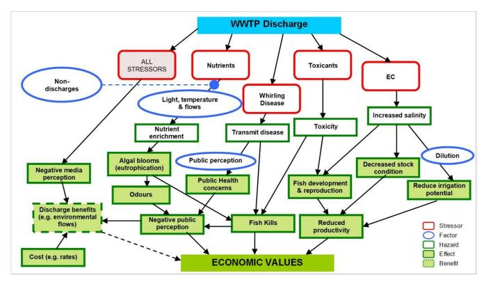
Figure B6 – Conceptual model of the relationship between a wastewater treatment plant (WWTP) discharge and the economic values of the Goulburn River. Notes: EC = electrical conductivity
