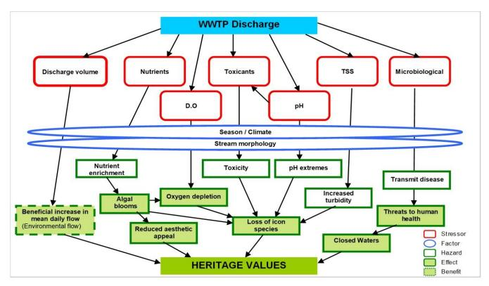
Figure B5 – Conceptual model of the relationship between a wastewater treatment plant (WWTP) discharge and the heritage values of the Goulburn River. Notes: D.O = dissolved oxygen, TSS = total suspended solids
