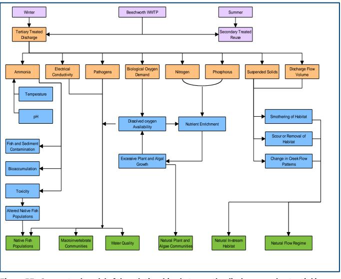
Figure B7 – Conceptual model of the relationships between the discharge and potential issues influencing water quality and ecological conditions in the Spring and Reedy creek systems
