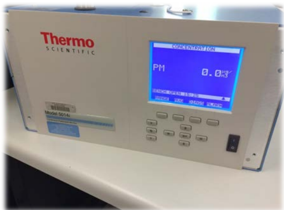
Figure 5: A BAM instrument that measures airborne particles (PM 2.5 ).
