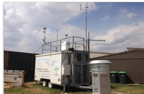
Figure 2: One of the 'local conditions' monitoring stations, which contains a beta attenuation monitor (BAM).
