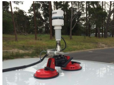
Figure 1: One of the mobile, rapid-response air monitoring devices used by EPA during the Hazelwood mine fire. The pictured device shows the inlet for a DustTrak™ instrument.
