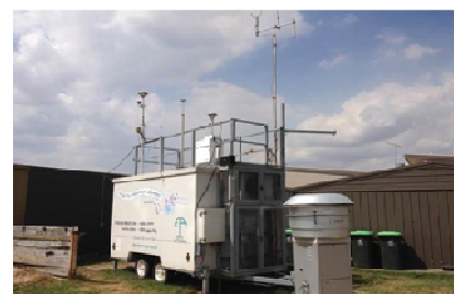
Figure 2: Air quality station housing a BAM - two of these stations were installed in Morwell during the Hazelwood mine fire.
