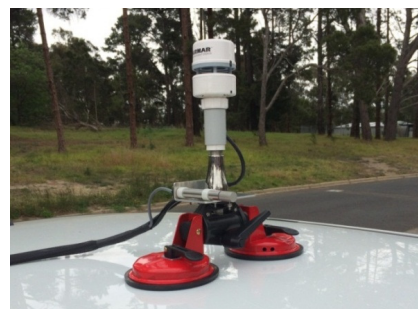
Figure 1: The inlet for a DustTrak™ instrument - a number of these rapid-response monitoring instruments were used by EPA during the Hazelwood mine fire.
