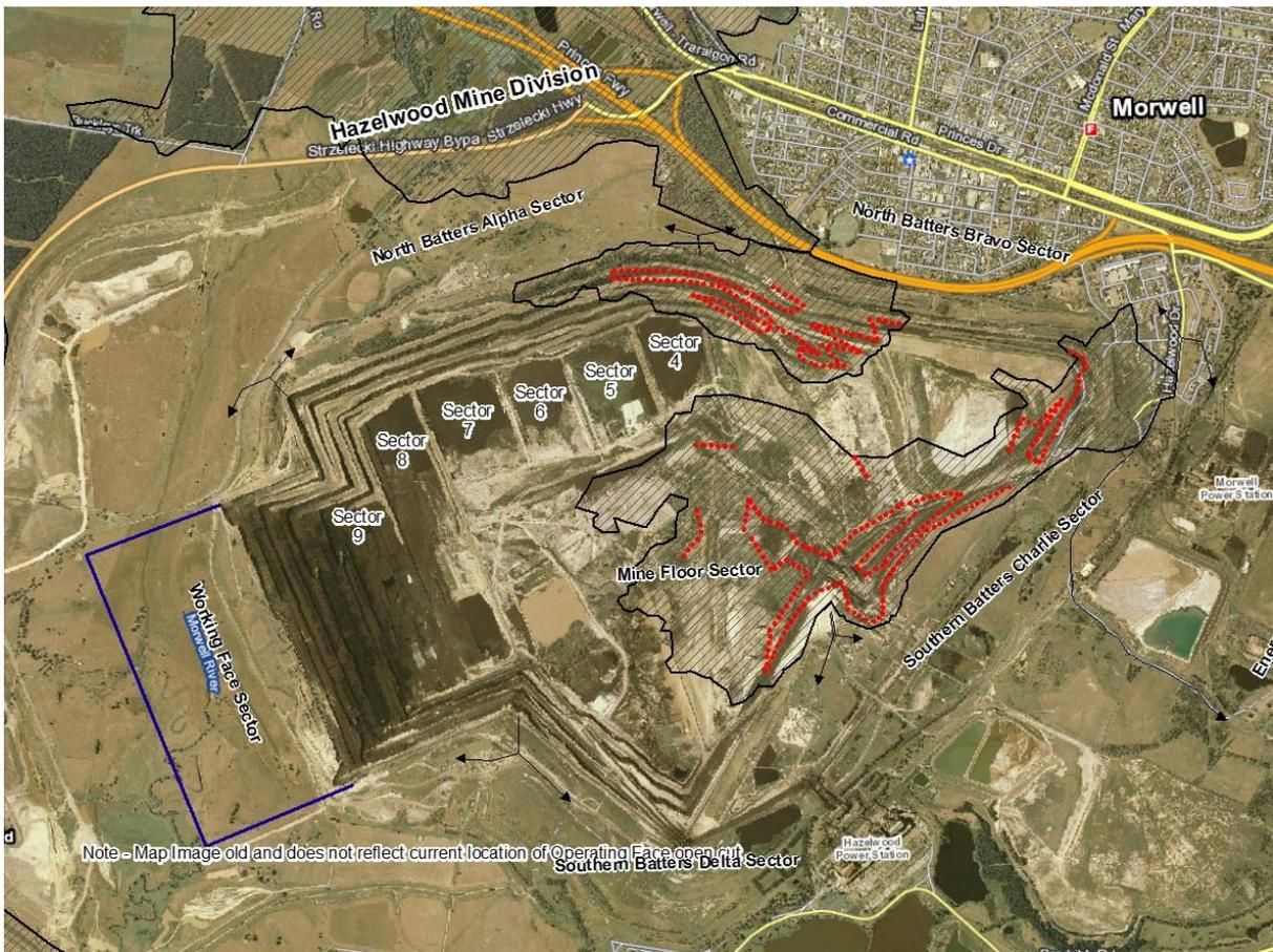
**Figure 4 Map of the Hazelwood mine. Red colour indicates the batters on fire.**
