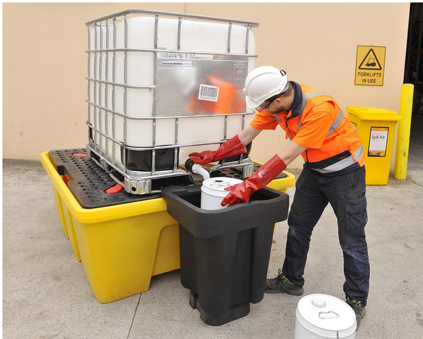
Figure 12: An intermediate bulk container (IBC) on a spill pallet with a dispensing unit attached. The spill pallet reduces the risk of leaks or spills from the IBC while the dispensing unit directs any potential spills during decanting into the sump.
