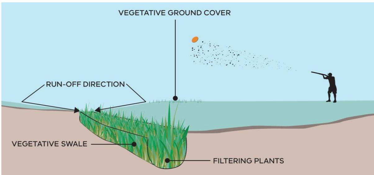
Figure 9. Simple water filtration system.
