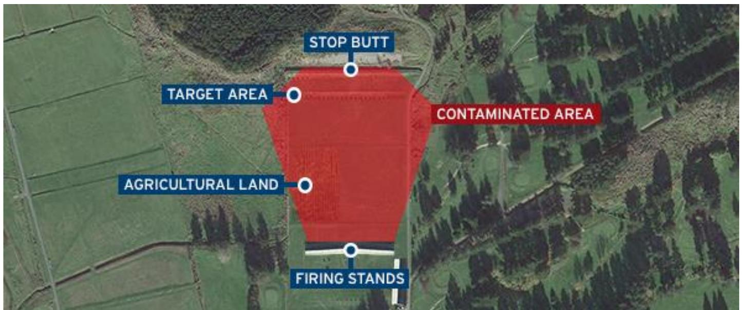
**Figure 3. Example of direct pathways at a rifle/pistol range.**
