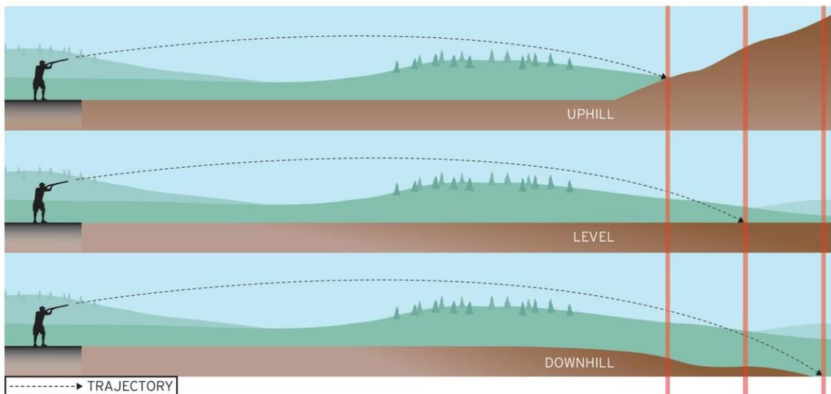
**Figure 14. The effect of slope on the distance shot travels.**
