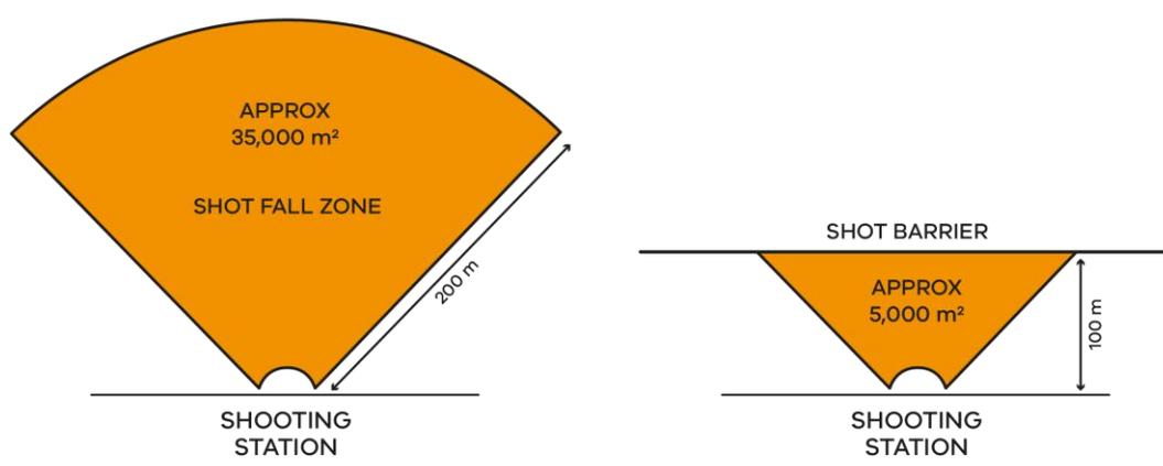
**Figure 15. Reduction in the shot fall zone by using a barrier at a trap station.**
