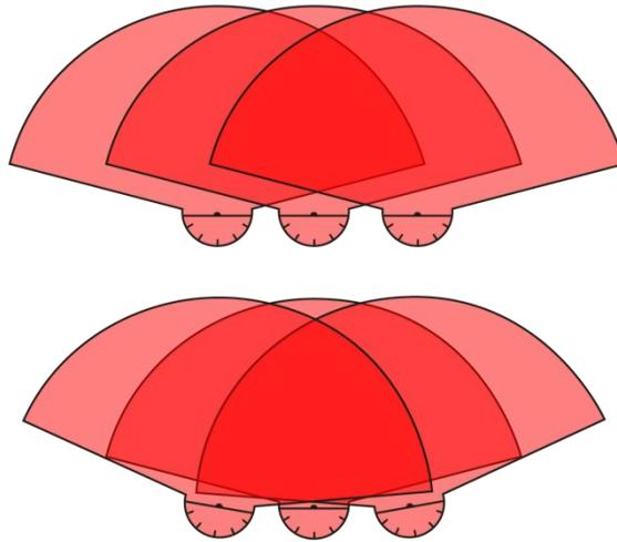
**Figure 12. Using overlap to reduce shot fall zone at a Skeet Field.**
