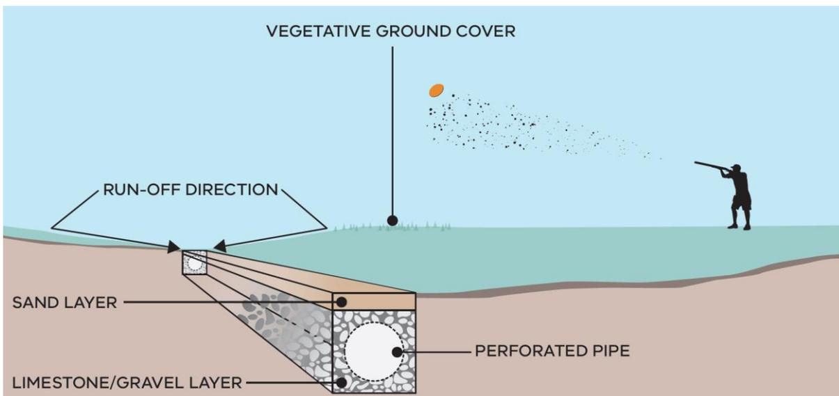
Figure 10. Advanced water filtration system.
