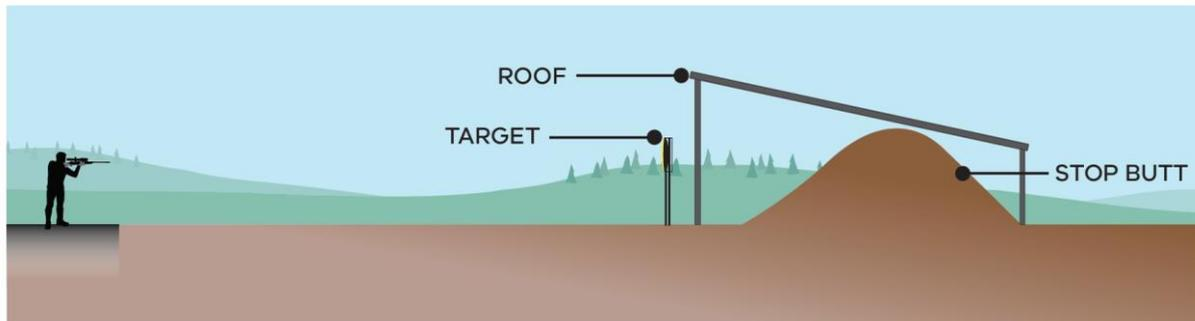
**Figure 17. Roof covering stop butt.**
