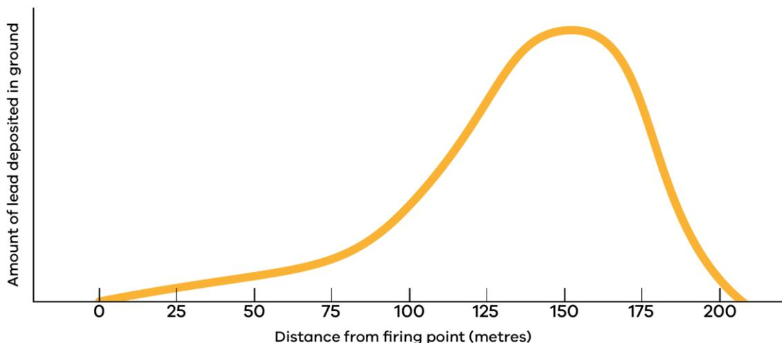
Figure 5. Lead contamination at a skeet or trap range based on distance from the firing point.
