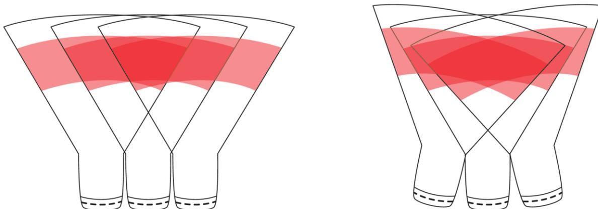
**Figure 13. Using overlap to reduce shot fall area at trap field.**
