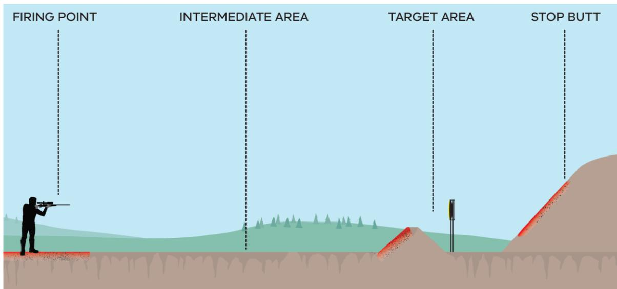
Figure 7. Contamination hotspot areas at a rifle or pistol range.
