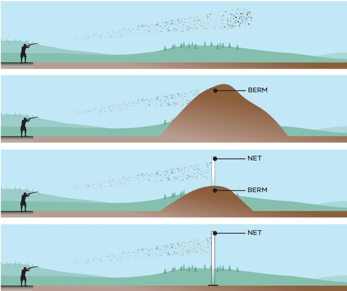
**Figure 16. How berms and nets can restrict the spread of shot.**
