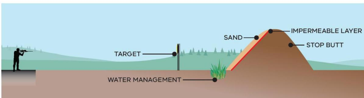
**Figure 18. Water management at the stop butt.**
