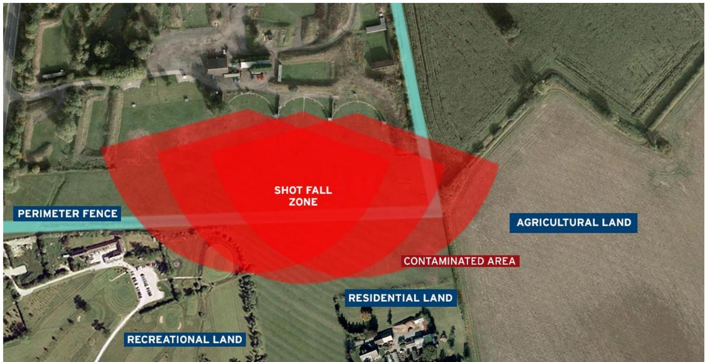
**Figure 2. Example of direct pathways at a shotgun range.**
