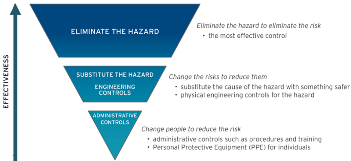
Figure 2: Hierarchy of controlling hazards and risks.
