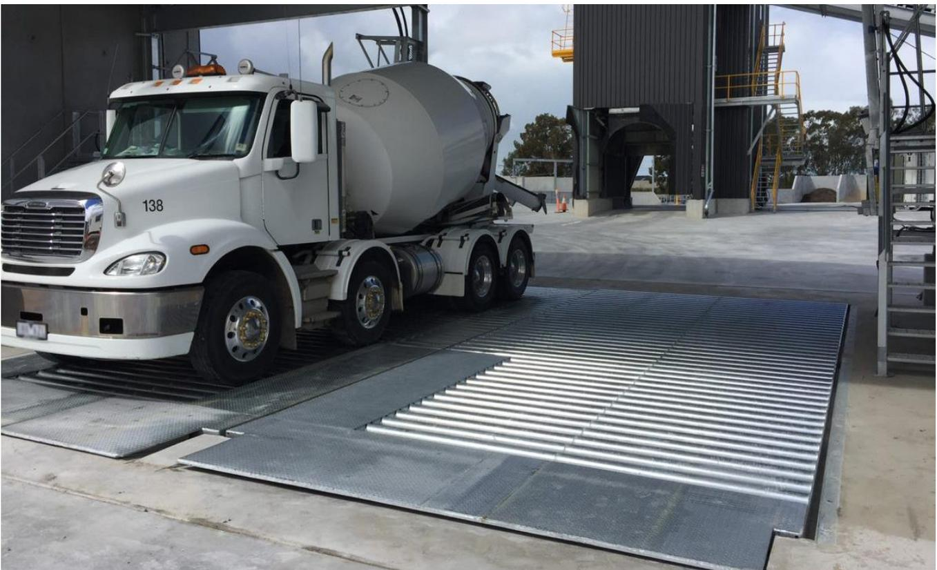
**Figure 6.** Slump station with grated floor to capture washwater for recycling back into production. *Source: Cement Concrete and Aggregates Australia (CCA).*
