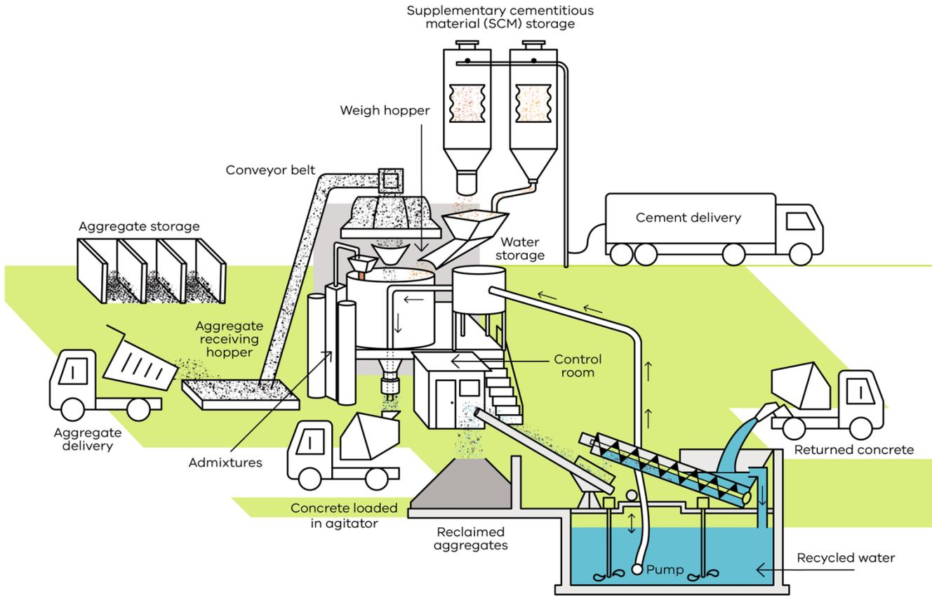
**Figure 1.** A flow-chart illustrating the concrete batching process. Adapted from Dr. Adel El Kordi, CVLE 519 Concrete Technology.
