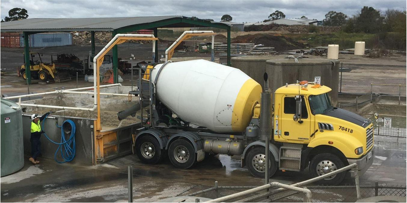
**Figure 8.** Waste concrete returned to batching plant for reclamation and recycling. Source: Cement Concrete and Aggregates Australia (CCA).
