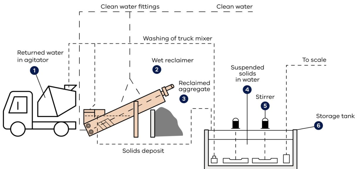
**Figure 9.** Example system for recycling washwater and aggregate recovery from fresh waste concrete. Adapted from: Kien, Tong., Le Thành., and Pham, Lanh. (2013). *Sustainability in the concrete industry for construction of mega cities*.
