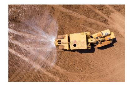
those with protected flora are sealed or actively treated with clean water to prevent dust. Some of their equipment that generates dust is kept in buildings fitted with extraction fans.
