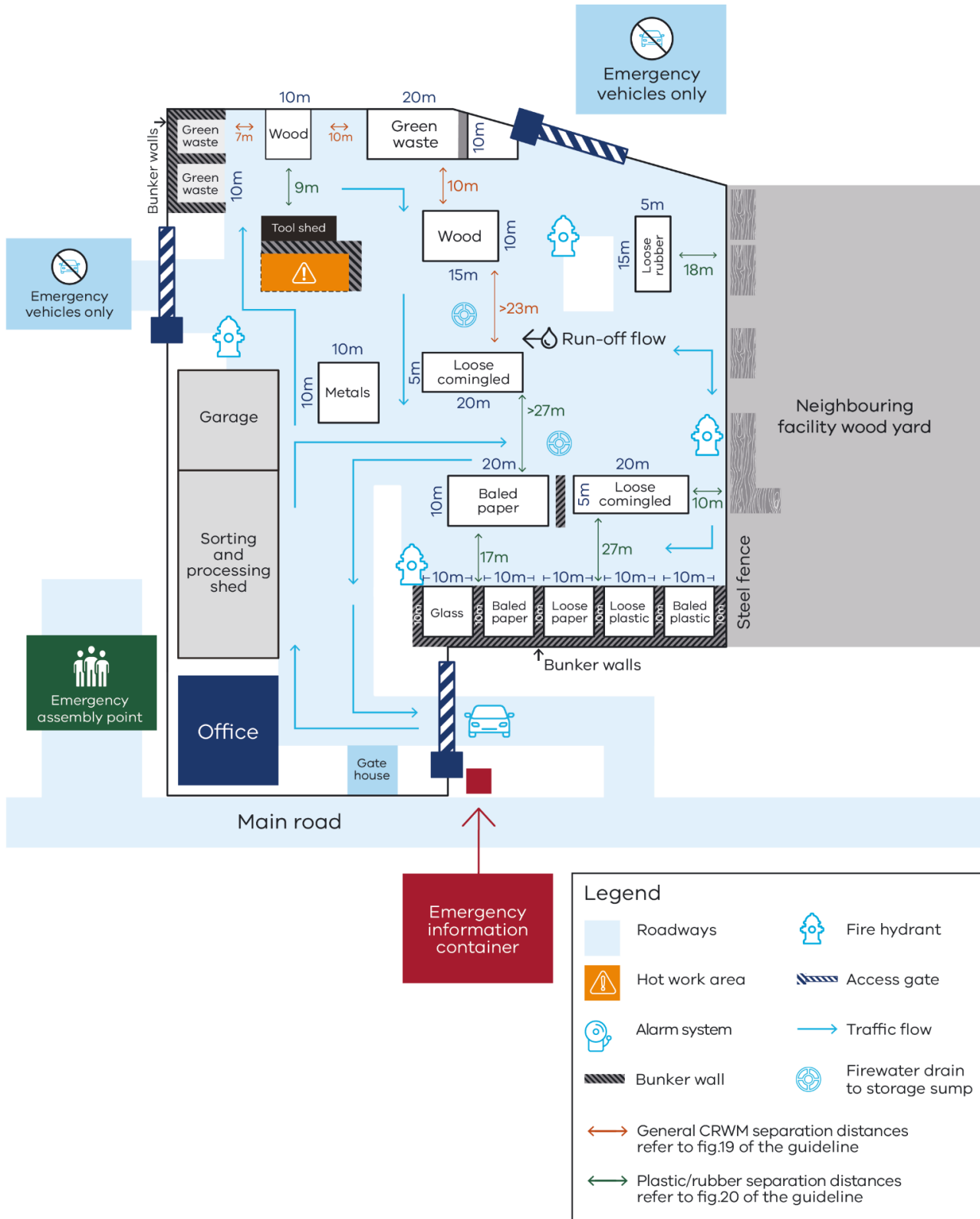
Figure 2: Nicole's facility after controls have been implemented. Note the figure is not drawn to scale.
