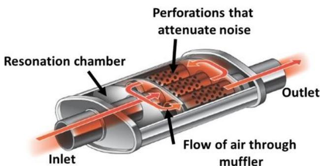
Figure 1. Design of a basic muffler.
