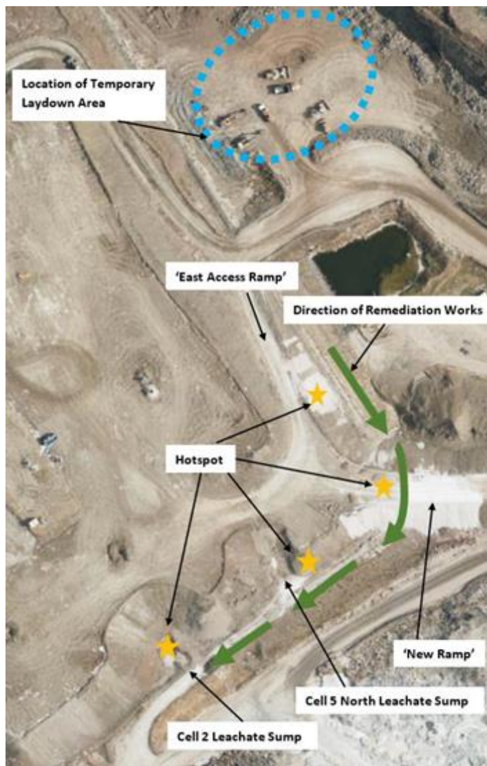
Figure 5: Proposed remediation works for Kealba landfill hotspots. Source: Golder report: Landfill hotspot remediation design, 27 March 2020, prepared for Barro Group.
