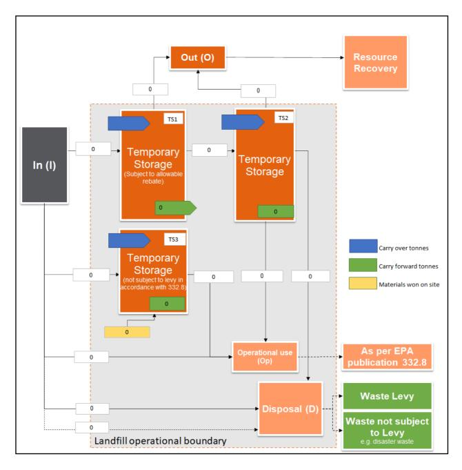
Figure 1 Waste flow diagram for mass balance calculations
