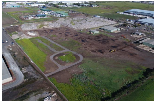
The Broderick Road site in April 2020, after the removal of 26,600m 3 of timber and 7,600m 3 of soil
