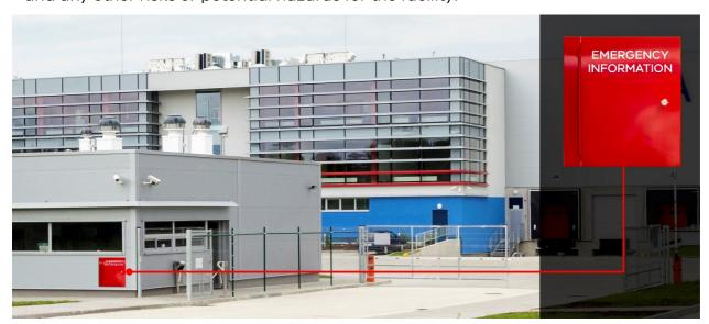
Figure 22: The Emergency Information Container (EIC) should be located at your site as close as reasonably practicable to all vehicle entrance(s).
