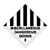
The Class label must not be less than 250 mm square and must be firmly affixed to the vehicle.
